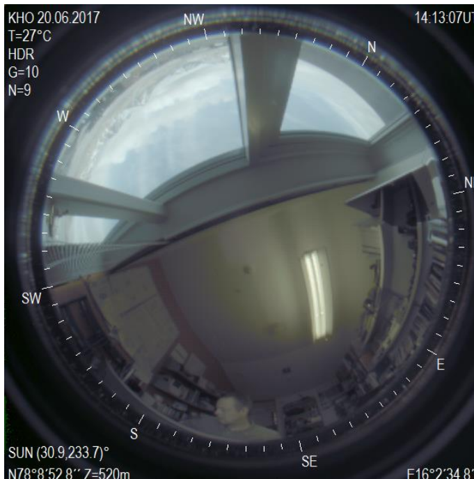
Figure 14. High Dynamic Range (HDR) imaging. Left panel: ASI174MC-Cooled camera response function. 16 Right panel: Office view HDR image constructed with 9 exposures at 1, 3, 7, 10, 50, 100, 200, 300 and 500 ms. The gain was set to 0. The aperture of the Fujinon lens was set to minimum F/16.
