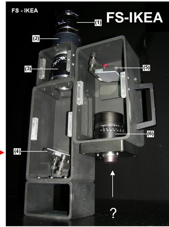
Figure Caption: The FS - IKEA. (1) front lens, (2) slit house, (3) collimator lens, (4) flat surface mirror, (5) blazed grating, and (6) camera / detector lens.
