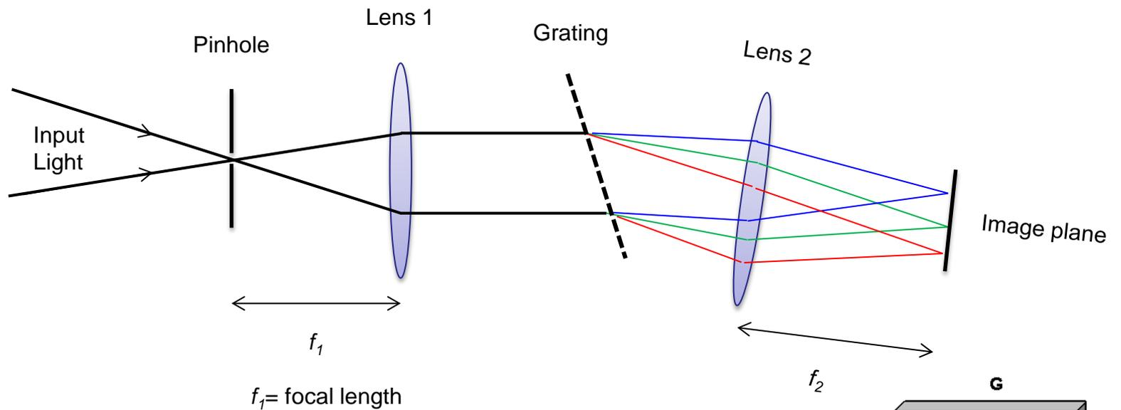
The result is a Grating spectrograph. It diffracts opposite in color compared to the prism spectrograph.
