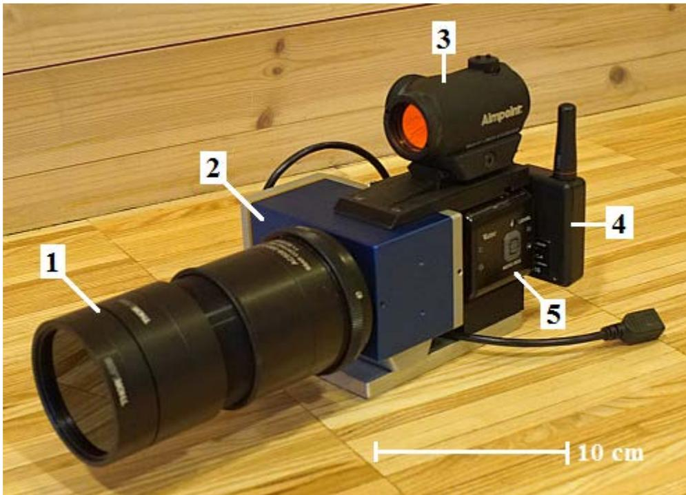
Prototype hyperspectral camera: (1) lens, (2) Liquid Crystal Tunable Filter (LCTF)- Varipsec, (3) aimpoint, (4) radio controller of camera head, and (5) Astrovid camera head.
