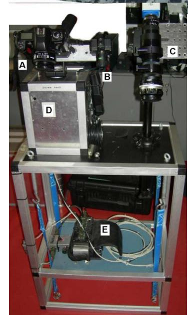
(A) S2Pro DSLR, (B) Webcam, (C) Hyperspectral imager, (D) Gyro / INS & (E) Battery pack
