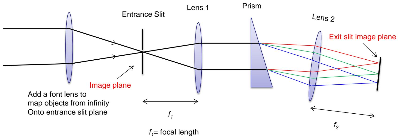
We now have an image in the entrance slit plane of the spectrograph. But only a slice of this image is allowed to enter. This slit image slice is now seen as a function of color in the exit plane. This will create structure in the spectrogram in the parallel direction of the slit.
