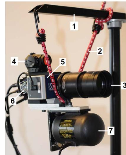
Gyro rig: (1) mount arm, (2) elastic rope, (3) lens, (4) aimpoint, (5) Varispec filter, (6) camera head, and (7) hand held gyro stabilizer.
