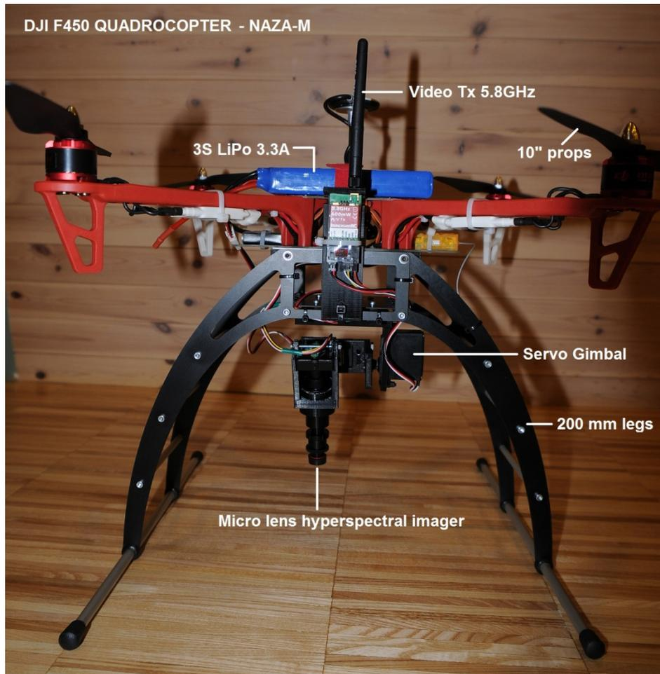
Instrument mounted to a DJI F450 Quadcopter.
