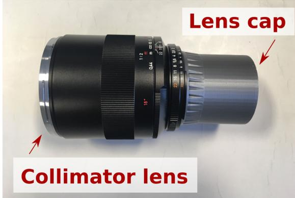
Figure 3.5: The collimator set-up consisting of a Zeiss Makro-Planar 100 mm f/2 lens, and a 3D printed lens cap with top pattern.
