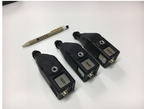
Figure 1: Three out of ten serial produced Hyper Spectral Imagers (HSI) version 4 by Moon Labs .
