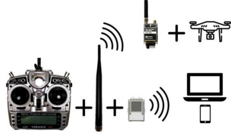
Figure 15: The general communication structure of the RF Design RFD 900x TXMOD v2 setup [35].
