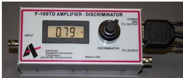
Figure 5. The F-100TD Preamplifier / Discriminator from Advanced Research Instrument Corporation with trimmed threshold control.
