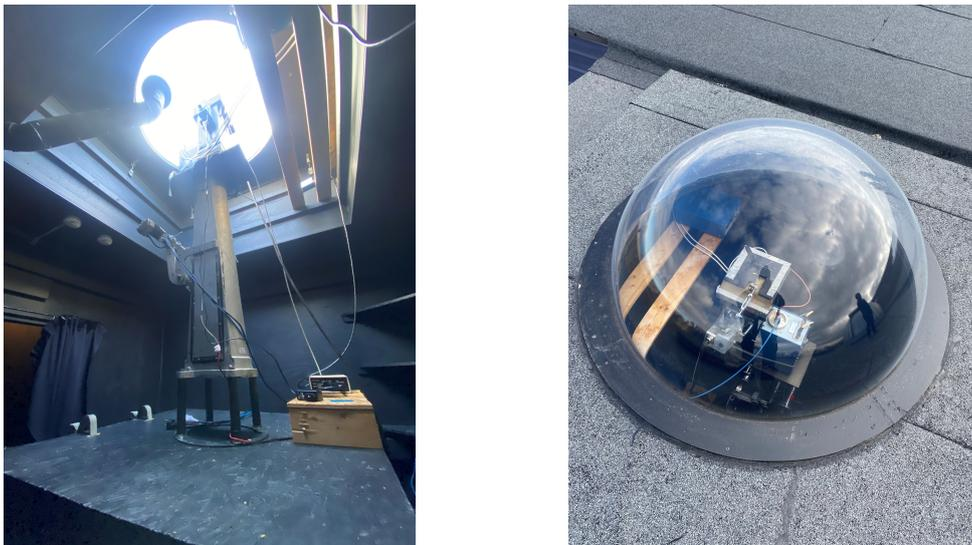
Figure 2: The 1m Ebert-Fastie spectrometer, "Silver Bullet"
