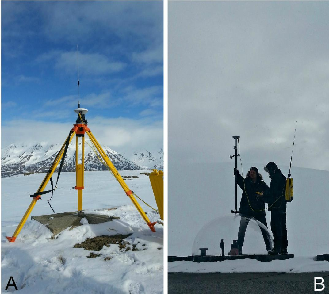
Figure 6.1: Panel A: The DGPS station placed over the marked location in Svalbard, nearby KHO. Panel B: The centre of each dome on the roof of the observatory is measured with the user equipment communicating with the DGPS reference station.
