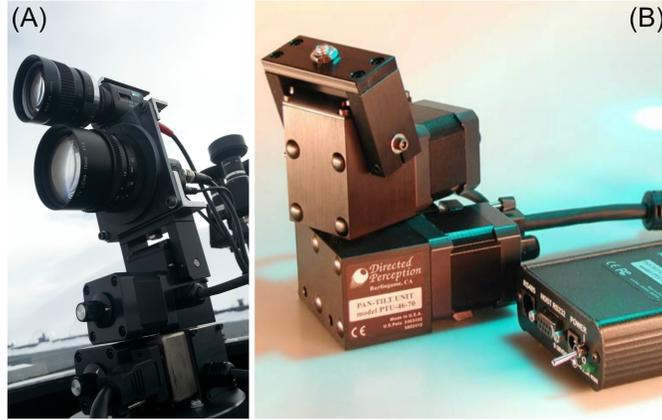
Figure 3.3: The PTU D46 platform. Panel (A): Example for the use of the PTU D46 unit at KHO: the instrument Tracker Camera. The Watec LCL-217HS is mounted on the top, while the Watec 902B is the bottom camera. Panel (B): The PTU D46 unit with its motor controller. Image from Directed Perception (2007).
