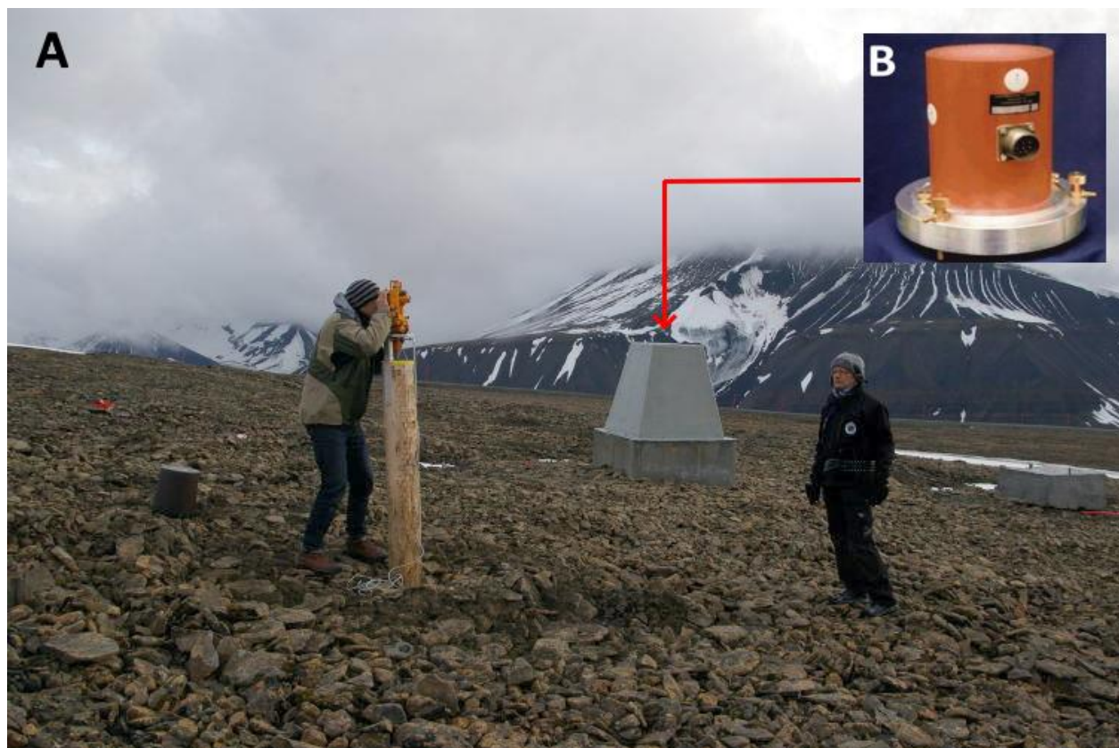
Figure 5. The Fluxgate magnetometer. (A) Left: Senior engineer Børre Heitman Holmslet calibrating the magnetometer at the Kjell Henriksen Observatory (KHO). Middle: Concrete base construction with protecting cover for sensor head. Right: Prof. Chris Hall (1953-2021) overseeing the operation. (B) Fluxgate sensor head.
