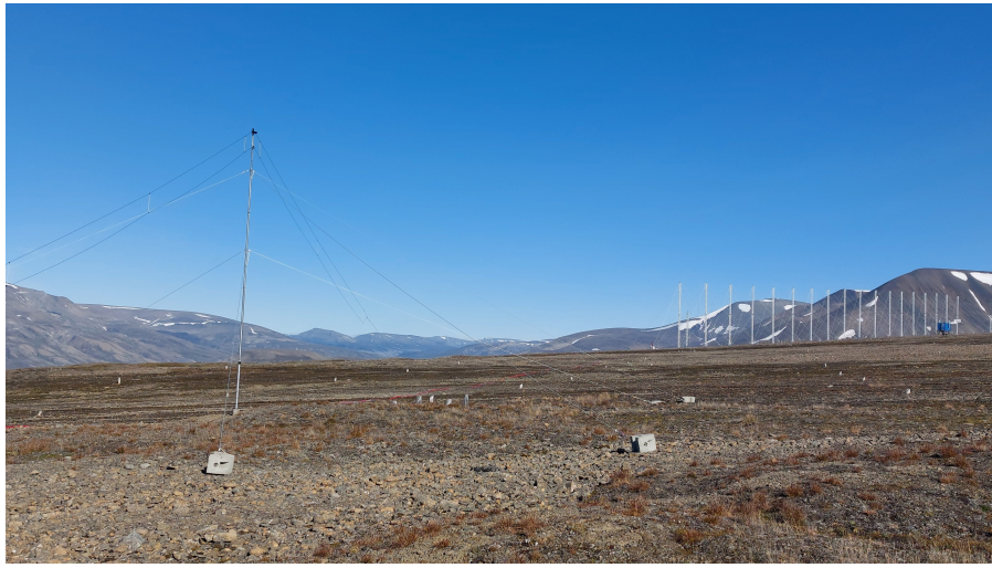
Figure 14: Picture of the transmitter antenna at SPEAR, with SuperDARN in the background
