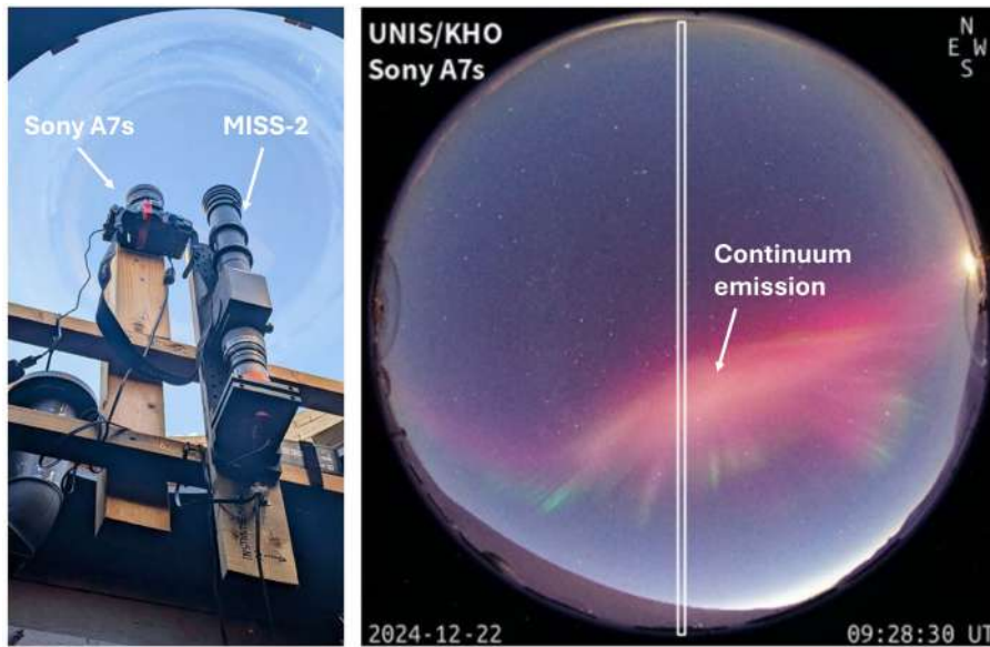
Figure 3.2: (Left) Image from inside the dome located on the roof of the Kjell Henriksen Observatory that hosts the Sony A7s all-sky camera and Meridian Imaging Svalbard Spectrograph (MISS-2). (Right) Image taken by the Sony A7s camera on 22-12-2024 at 09:28:30 UT. The white rectangle indicates the field of view of MISS-2 along the magnetic meridian.
