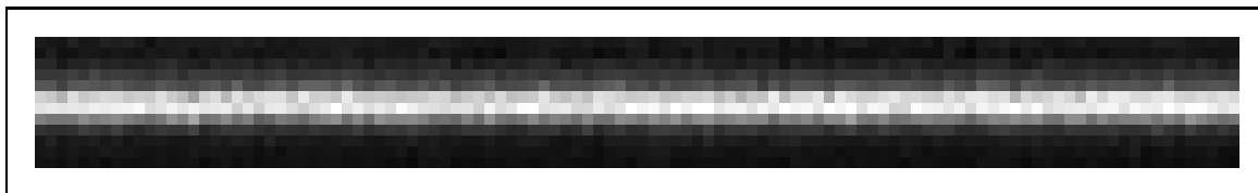
Figure 5.8: Slice through the center of the image of the point source (vertical dimension) showing pixel jitter as a function of time (horizontal dimension). The centroided locations are quantified in Figure 5.9.
